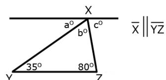
Angle  $a$  is  $35^\circ$  because it alternates with the angle inside the triangle that measures  $35^\circ$ . Angle  $c$  is  $80^\circ$  because it alternates with the angle inside the triangle that measures  $80^\circ$ . Because lines have a measure of  $180^\circ$ , and angles  $a + b + c$  form a straight line, then angle  $b$  must be  $65^\circ$  ( $180 - 35 + 80 = 65$ ). Therefore, the sum of the angles of the triangle are  $35^\circ + 65^\circ + 80^\circ$
